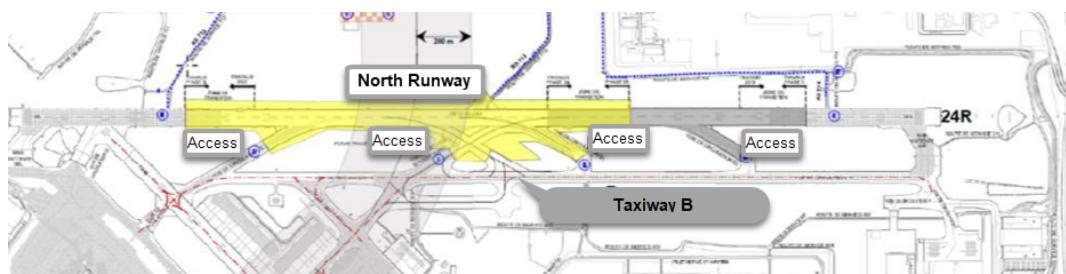
The work for this phase consists of building new concrete slabs on the central section of the runway that is still in asphalt as well as the associated electrical works. The reconstruction of 2 access roads to access the north runway (excavation of the existing surface, reconstruction of the infrastructure and asphalt surface) is scheduled as well as the completion of work started in 2022 on another access road.
